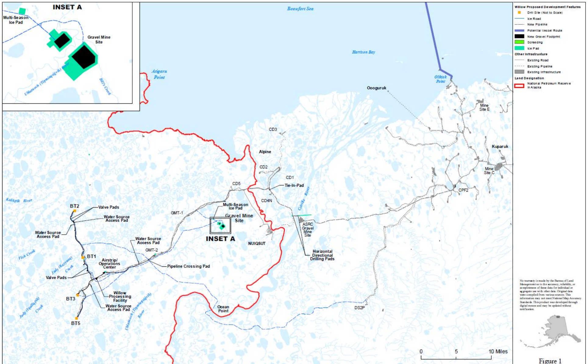
Figure 2.1. Overview of the proposed Project in northeast NPR-A, including permanent (gravel) and seasonal infrastructure, existing Kugaruk Unit infrastructure east of the Colville River, and Oliktok Dock.
